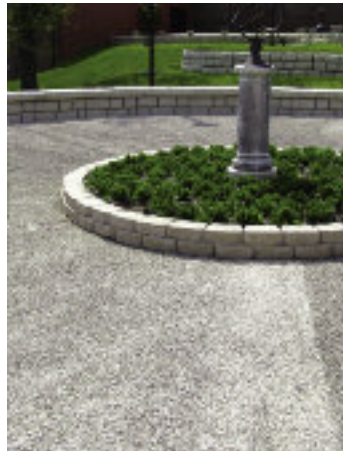
Permeable concrete was used for the McKown Plaza at Shenandoah University.
