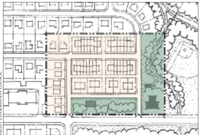
Cluster – 48 dwelling units (reflecting a bonus) in a mixture of unit types. The historic house and the stream valley are preserved (30% open space).
