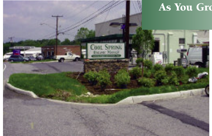
Before and After: A “low-impact development” project in Lexington added rain gardens for better stormwater management and an attractive gateway.
